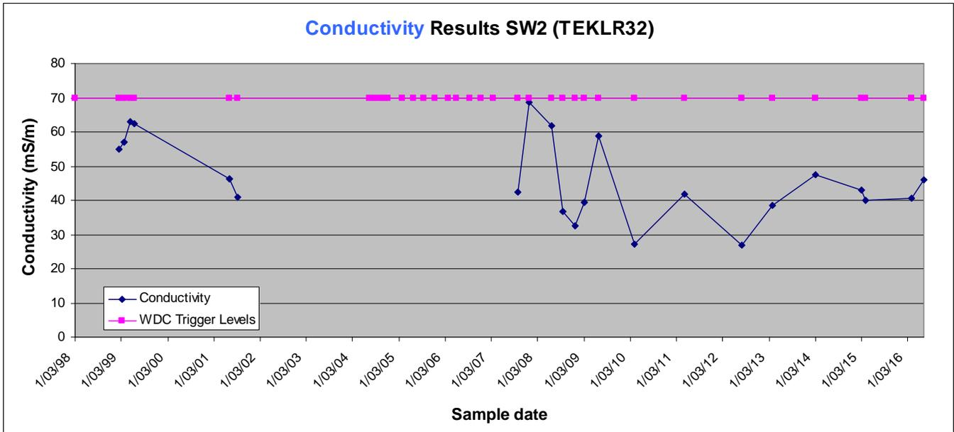
**Figure 2:** Waitomo District Landfill SW2 conductivity results from March 1998 to July 2016 (the pink line indicates the WDC trigger level of 70 mS/m).
