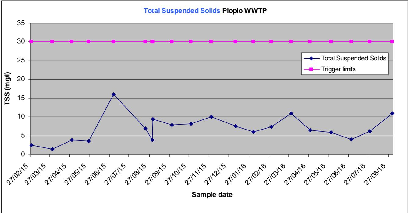
**Figure 4** – Total Suspended Solids Results Piopio WWTP
