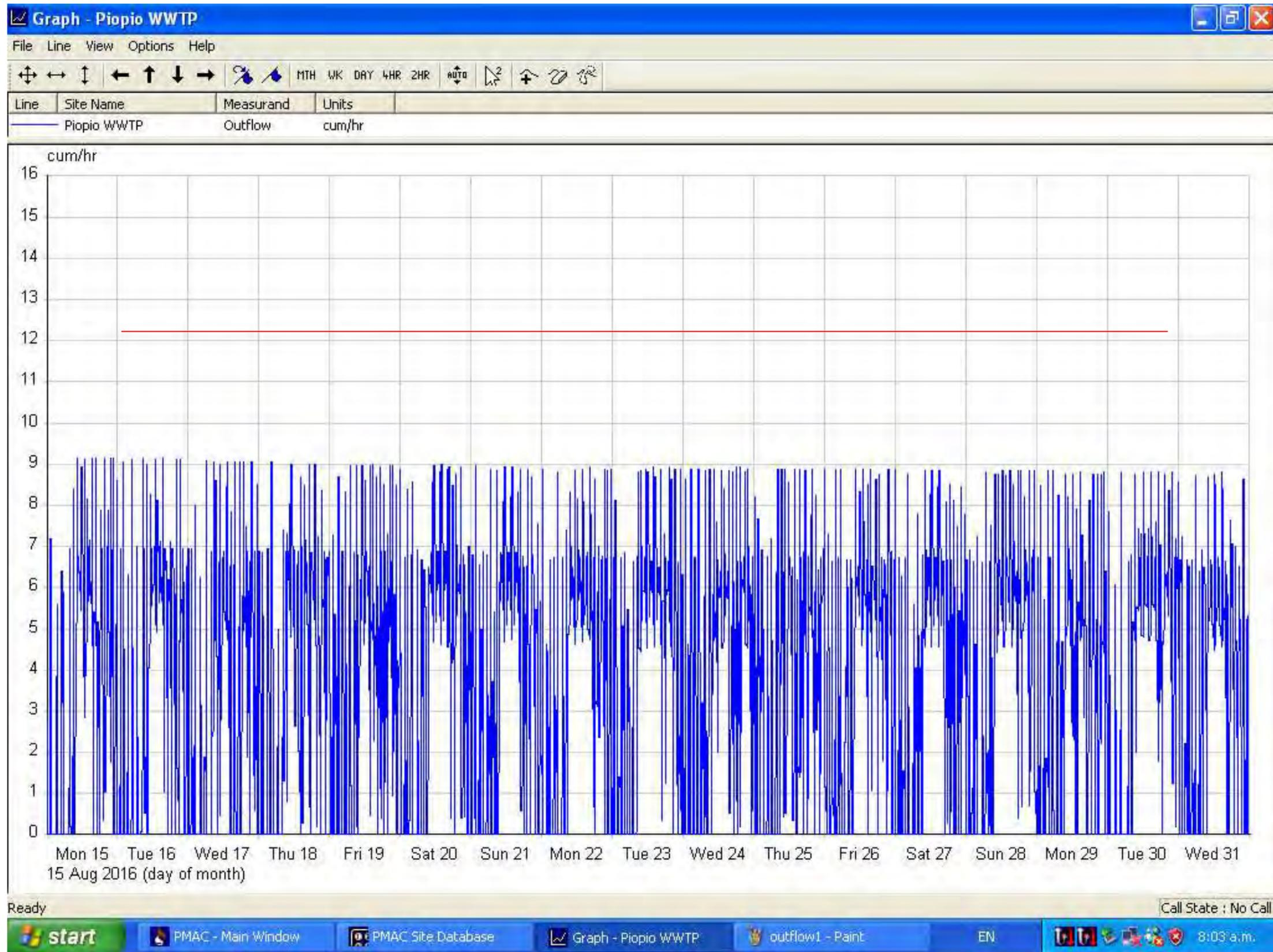
**Figure 8** – Discharge flow rate August 2016 ( $11 \text{ m}^3/\text{hr} = 3.05 \text{ l/s}$ )
