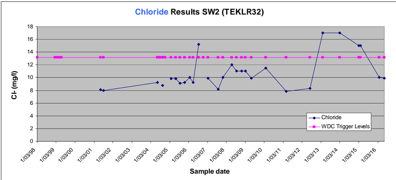
**Figure 3:** Waitomo District Landfill SW2 chloride results from March 1998 to July 2016 (the pink line indicates the WDC trigger level of 13 g/m3).
