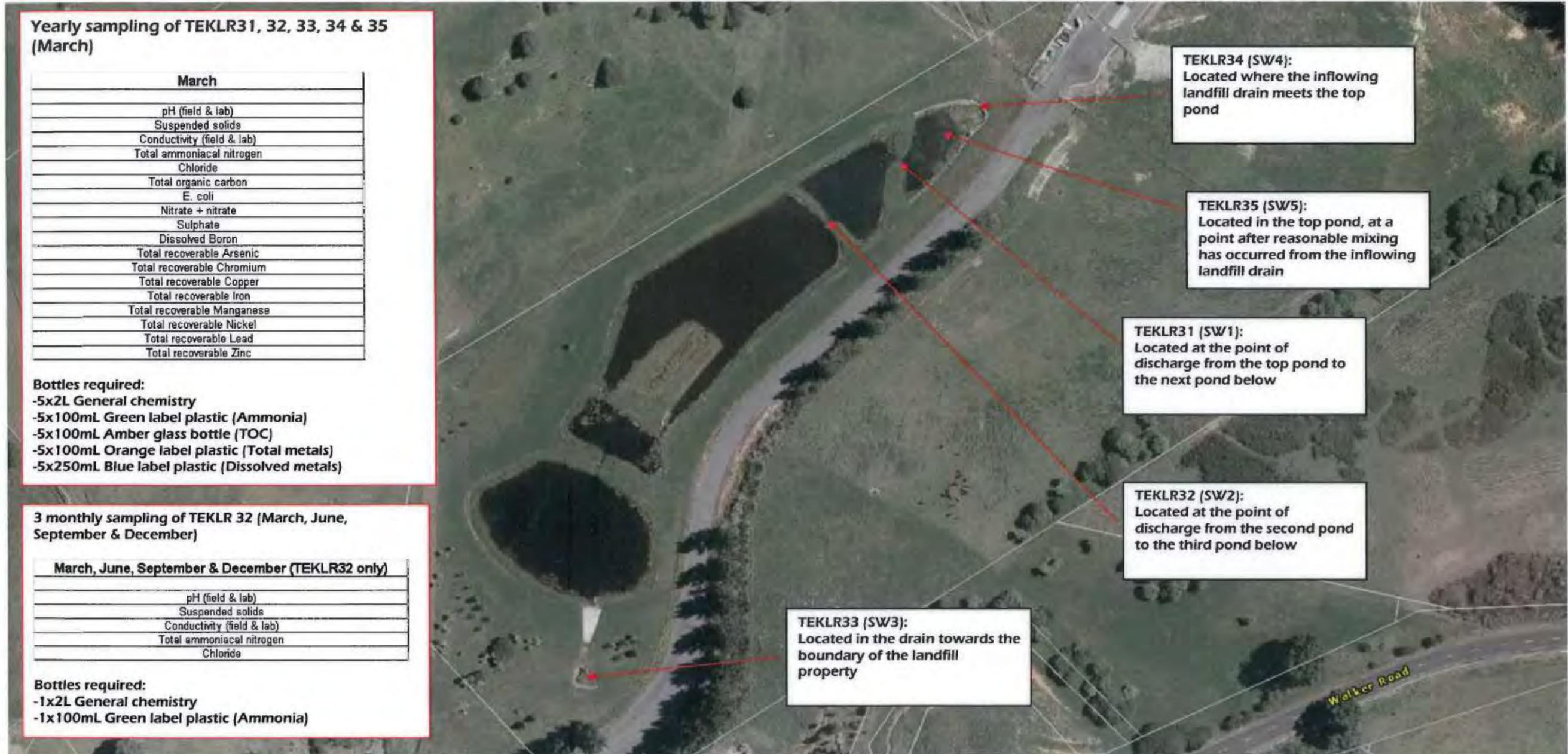
Figure 3 – WDC Proposed Map for Monitoring Sampling locations with reallocated sampling points SW4 and SW5.
