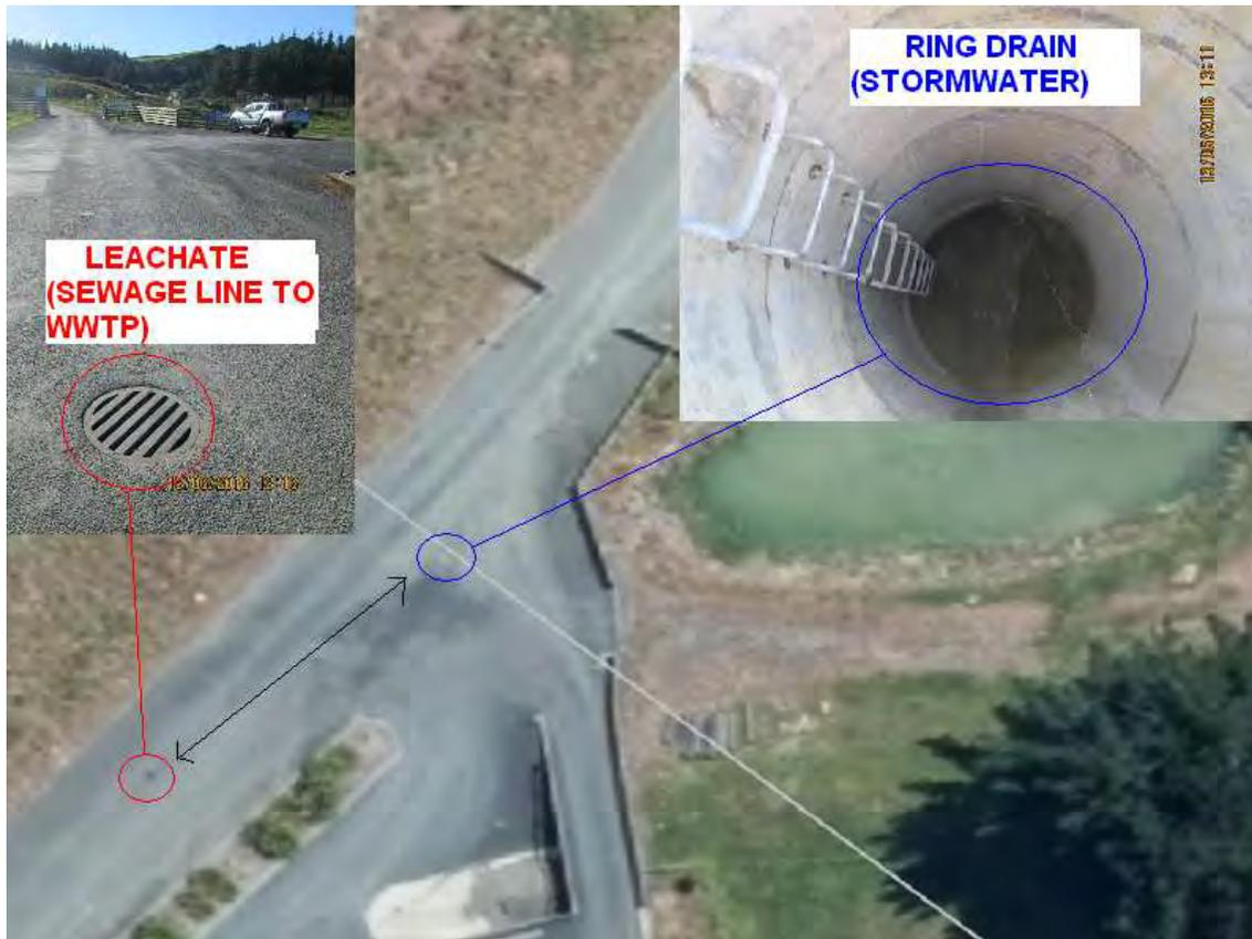
In previous years these two sampling locations have been accidentally swapped around during sampling, the confusion was probably because the manhole lid for the Ring drain was painted red (sewage) instead of white (stormwater) and the leachate sampling location has a grate with no colours or marks. This has been corrected and Contractor has been advised about the correct sampling points to avoid future incidents.
