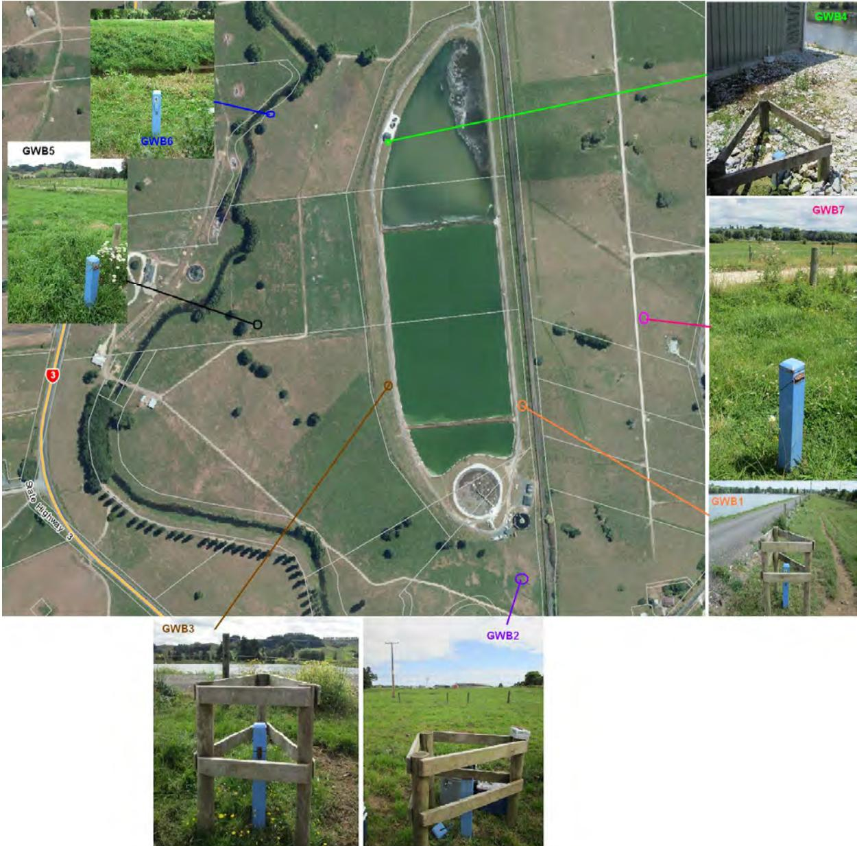
**Figure 1 – Bore locations** - The Te Kuiti WWTP is located approximately 2Km north of the Te Kuiti Township. The plant consists of a primary settling pond, clarifier and two oxidation ponds. Treated effluent from the plant is discharged into the Mangaokewa Stream. The WWTP is located in an agricultural area and is bound by the North Island Main Trunk Railway Line to the east and
