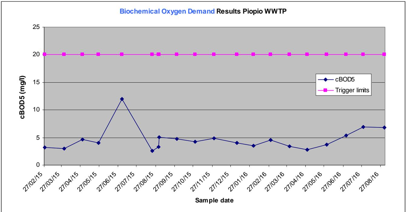
**Figure 5 - Biochemical Oxygen Demand Results Piopio WWTP**
