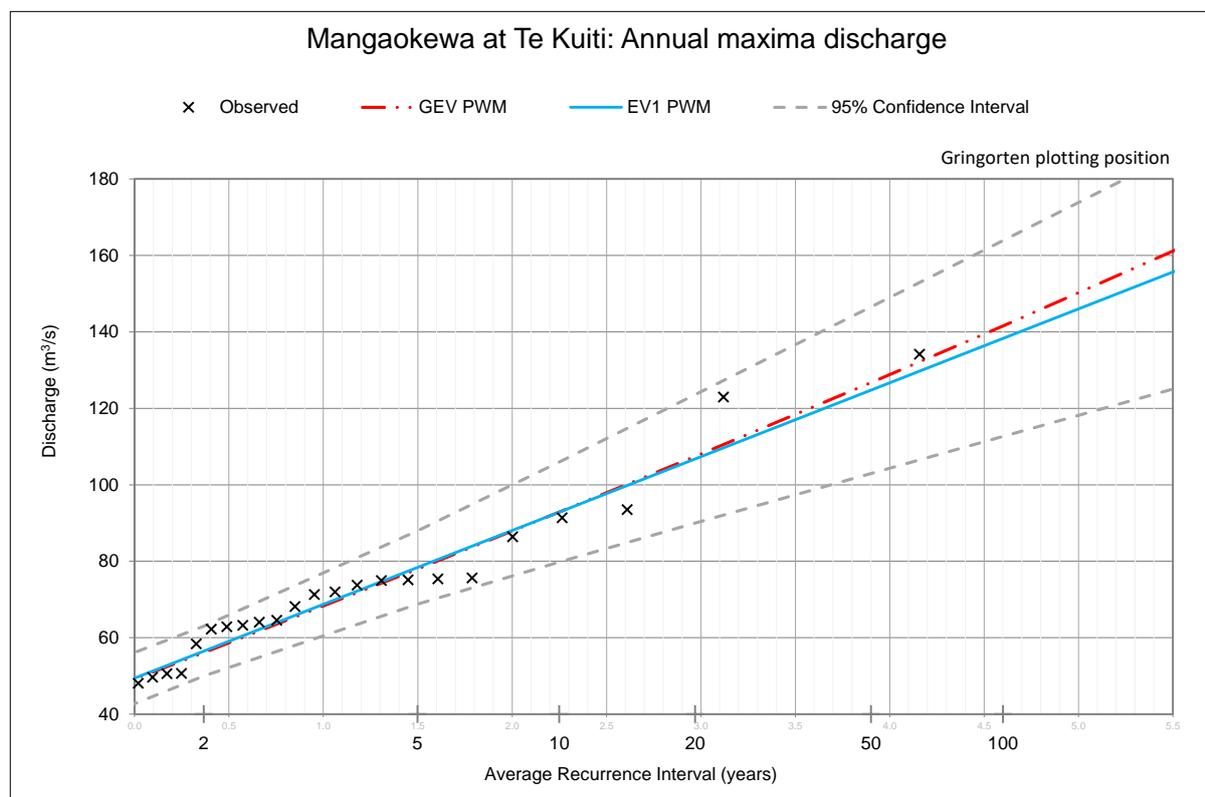
Figure 3.2: Mangaokewa at Te Kuiti: Flood frequency distribution
