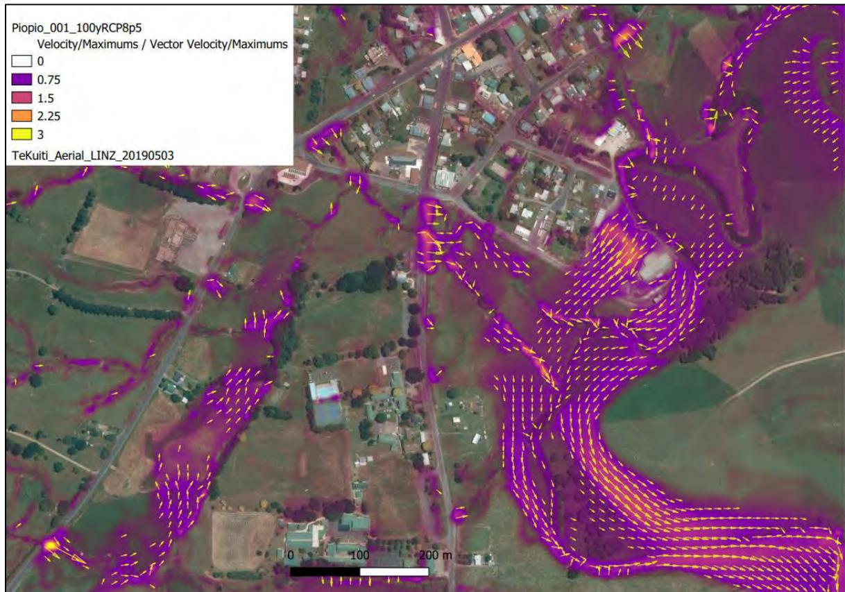
Figure 5.2: Sample maximum flood velocity output
