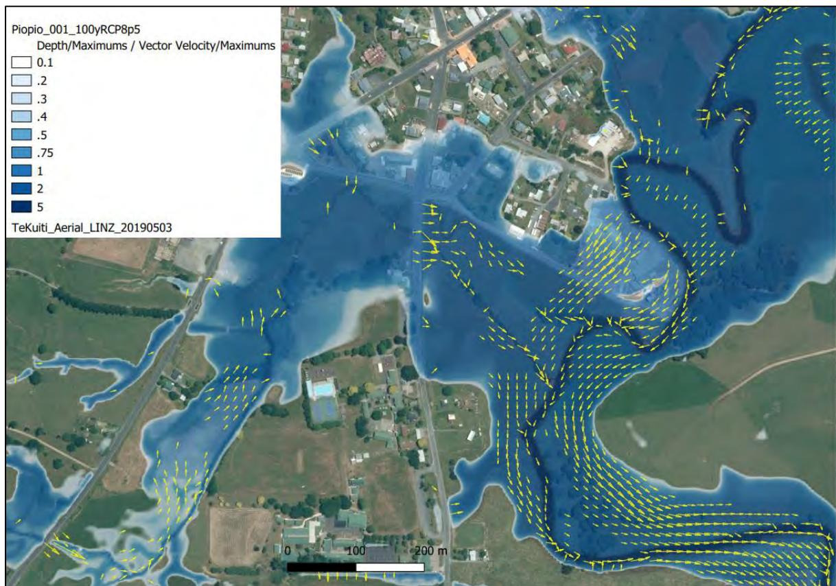
Figure 5.1: Sample maximum flood depth output
