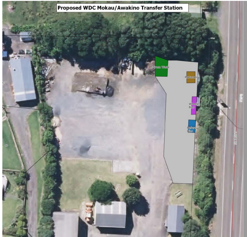
Figure 2: Proposed layout of Transfer Station showing greenwaste, portacom, wheelie bin, and refuse bin locations
