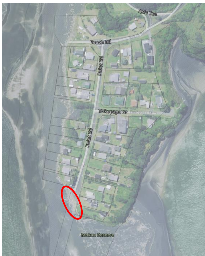
Figure 1. Mokau Spit showing location (red outline) of current 60m (approximately) long Point Road Seawall for renewal (Option 1) or removal (Option 2).
