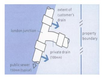
Figure 3–Typical Stormwater Connection.
