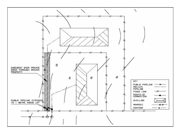
NB: While wastewater pipelines are depicted above, the same provision applies to stormwater pipelines
