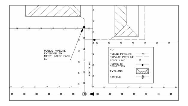
NB: While wastewater pipelines are depicted above, the same provision applies to stormwater pipelines.
