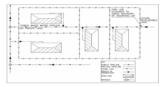
NB: While wastewater pipelines are depicted above, the same provision applies to stormwater pipelines.
