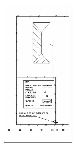
NB: While wastewater pipelines are depicted above, the same provision applies to stormwater pipelines
