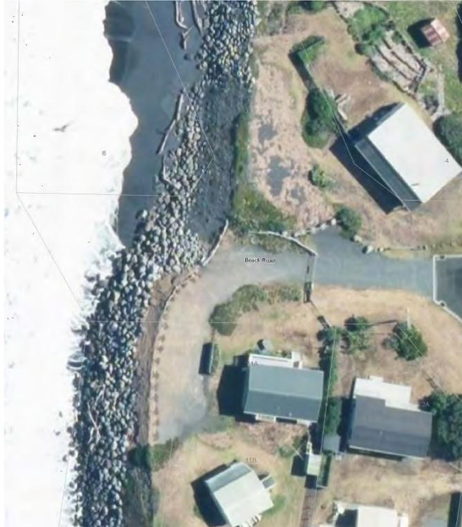
Photo 2: **TEMPORARY ROAD EROSION PROTECTION STRUCTURE, BEACH ROAD, MOKAU; 2015**
